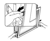
3. Push and close the top part of the front panel and then pull the bottom part of the panel forward until it is secured.
